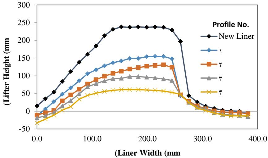
Figure 8. Wear profiles of a liner after 6200 h of operation at four points along length of liner.
