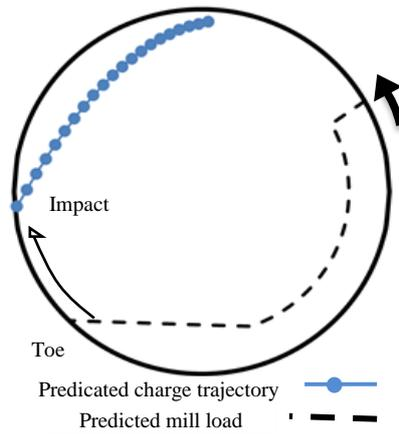
Figure 4. Simulation of 125 mm ball trajectory at 18% filling for old liner using GMT software.
