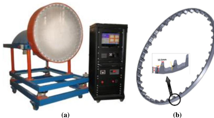
Figure 1. a) Model mill along with control and data acquisition system, b) polyurethane ring machined to scale down liners arrangement of an industrial mill.
