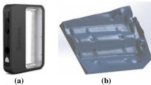
Figure 3. a) 3D scanner (Sense®) used in this research work, b) a typical snapshot of a scanned liner.
