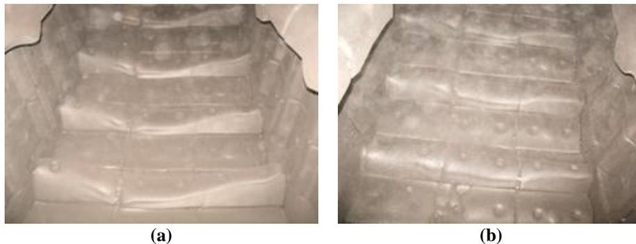
Figure 11. Snapshot of shell liners at end of life time; a) uniform liners (design No. 1), b) non-uniform liners (design No. 2).
