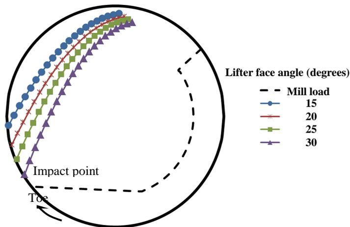
Figure 5. Simulation of 125 mm ball trajectories with different lifter face angles (24% filling).
