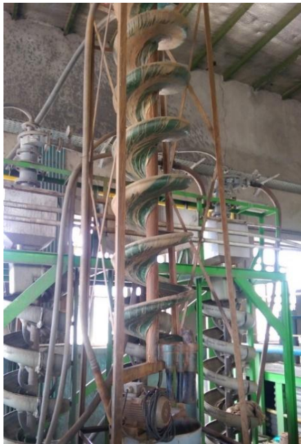
Figure 2. Pilot-plant spiral installed in a closed continuous system.
