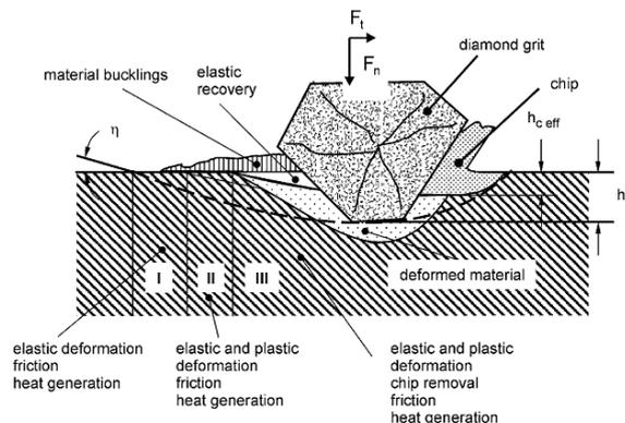
Figure 2. Cutting mechanism during grinding of metal material [14].
